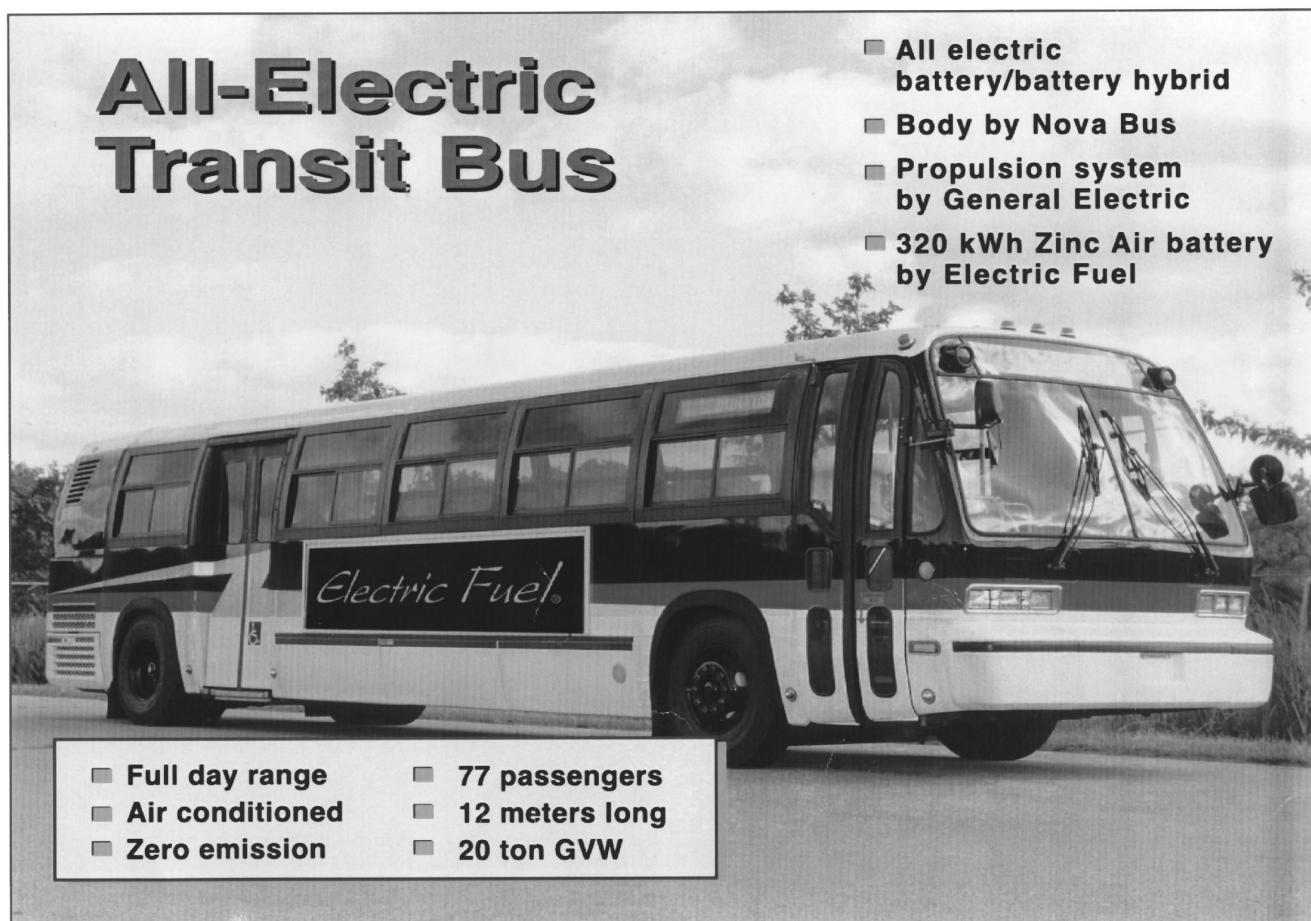
Fig. 6. The all-electric battery–battery hybrid demonstration bus.
