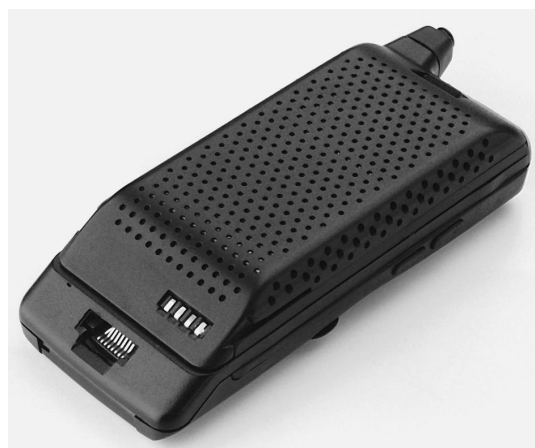
Fig. 8. Six-volt battery pack, with holes in the pack wall to allow air access to the zinc/air cell within, attached to a Motorola MicroTac handset.
